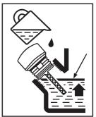
Please fill in the engine oil (approx. 0.55 l) until the oil level reaches the upper edge of the filler neck.
